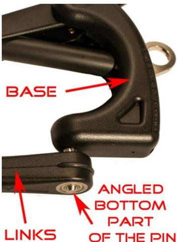
6. **ATTENTION!** Make sure the pin goes all the way through the links. The angled bottom part of the pin must come out underneath the links, like in the picture below. If this is not done correctly, the bearings might break.
